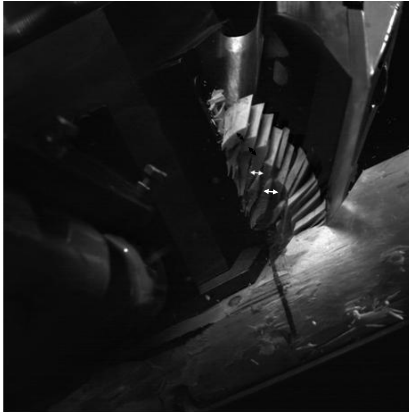
Figure 4. Fragmentation of an unfrozen log using a 448.7 mm cutterhead diameter combined with an attack angle of 85^\circ (infeed position: 199 mm). The black arrow shows a chip thickness that was defined by tangential ruptures and the white arrow shows a chip thickness that was defined by radial ruptures.
