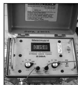
Fig 1: Aparelho Stress wave timer (SWT).
